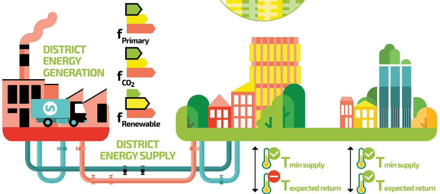
THE DISTRICT ENERGY INDICATOR INFORMS RESIDENTS ABOUT THE EFFICIENCY AND CLIMATE EFFECT OF THE NEARBY DISTRICT HEATING (OR COOLING) NETWORK. IT ALSO SHOWS WHETHER THE BUILDING CAN BE CONNECTED TO A LOW-TEMPERATURE DISTRICT HEATING GRID. OVERALL, IT PROVIDES AN INCENTIVE TO DECREASE CARBON EMISSIONS IN EXISTING DISTRICT ENERGY NETWORKS AND INCREASE INVESTMENTS IN NEW AND MORE EFFICIENT NETWORKS.
