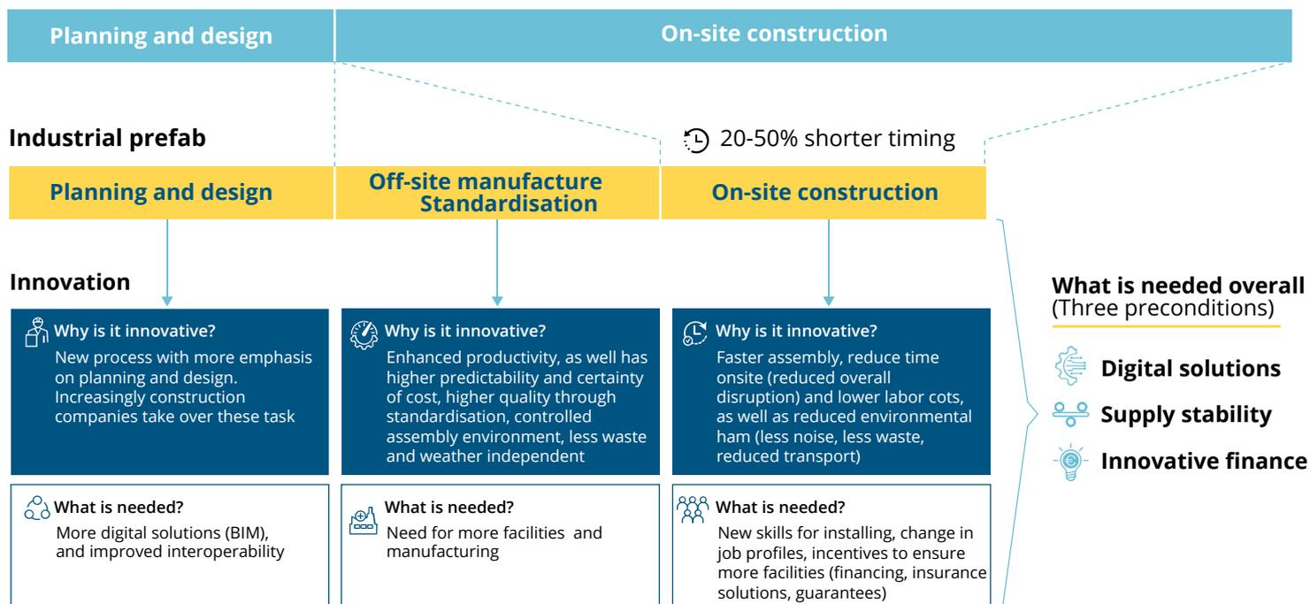
**Figure 1** - Traditional construction vs. industrial prefabrication (including innovation needs)
